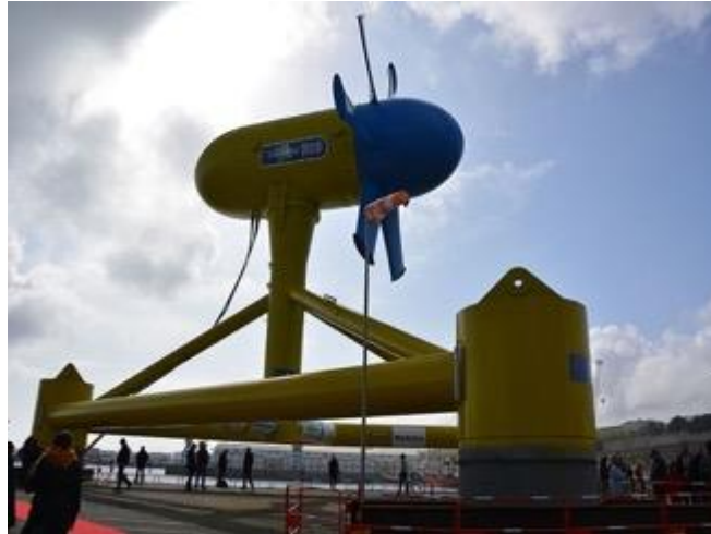
Figure 16 : Hydrolienne D10 Sabella (Source : http://blog.formatis.pro/sabella-d10 )
